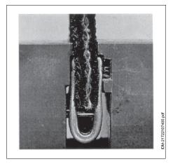
9. By using a hammer, introduce the punch into the left hole until its side touches the equipment. Hit the punch other 3 times to create the head of the nail.
