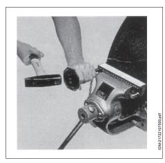
10.By using a hammer, introduce all nails into the belt (proceed from the right to the left).
