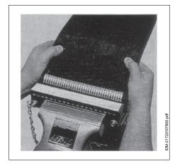
12. Crush the nails on a solid base.
