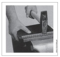
13.In case of belts having a different width, twist and remove the exceeding hooks.
