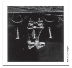
5. Before introducing the belt, tighten the vice until the junctions are slightly tightened and the belt can be easily introduced.
