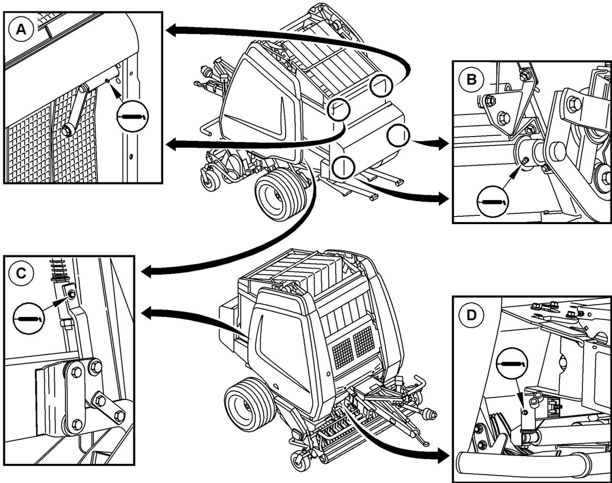
A—Bale Shape Indicator Arm    C—Gate Latch Rod Arms (862    D—Twine Arm Hub
