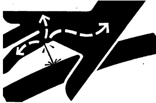
Always relieve hydraulic pressure before servicing hydraulic components.
