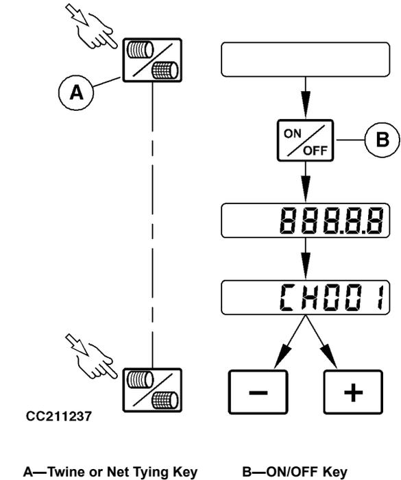
To return in normal mode and save the user parameters settings, switch OFF the monitor by pressing the ON/OFF key (B).
