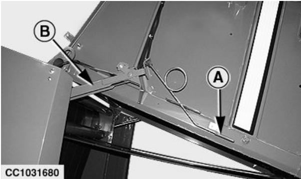
A—Lock device control lever      B—Gate lock device in locked position
