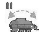
E94203—UN—12AUG20 Baler Ride Control On with Degraded Performance Icon (grey dashed arrow)
