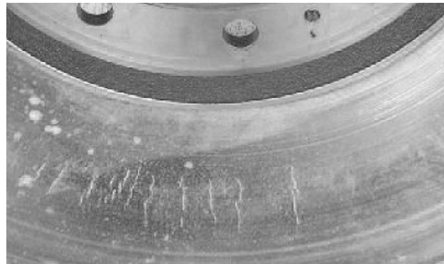
E72866—UN—20FEB14 Heat Checked Areas on Brake Drum
