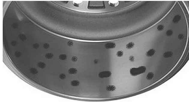
E72867—UN—11AUG14 Hard or Chill Spots on Brake Drum
