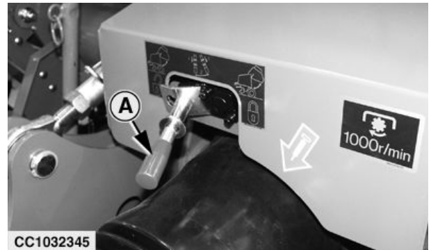
960 and 990 Gate Lock Device
