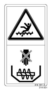
Never place your hand or an object near the augers when the engine is running.
