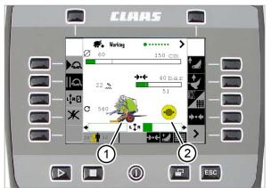
There is a graphical representation of the baling / tying process on the control terminal screen.
