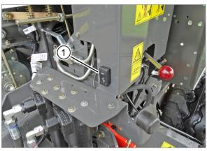
The work light is controlled by the switch (1).
