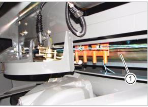
The twines must be in contact with the metal roller (1).
