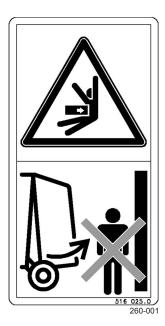
Stay outside the tailgate swing zone when the tractor engine is running.
