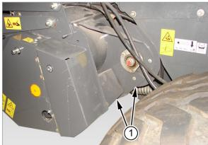
The pick-up is driven by the pair of gears (1) on the left-hand side of the baler.
