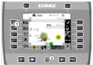
If the <ICT hydraulics> function is available on the tractor, and the tractor has been authenticated, the symbols (1) and (2) are displayed on the control terminal screen.
