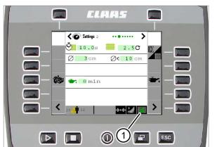
If the delay is set at 10 s, tying switches to <Manual tying> mode:
