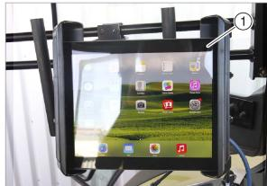
126 289447-001 The baler can be controlled directly using a touch tablet (Apple iPad) (1) if the tractor has an ISOBUS connection.
