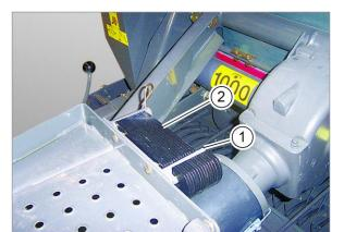
The knives (2) are fitted to the lower section of the dummy knife holder (1).
