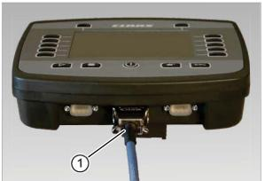
▶ Connect the flat connector (1) on the extension to the main connector on the COMMUNICATOR.
