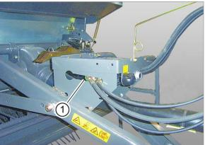
Slide the hydraulic hoses into the slot (1) on the step.
