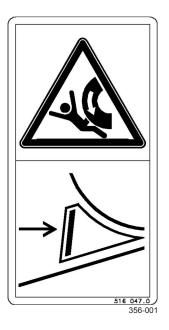
Before unhitching or storing the machine, secure it using chocks to prevent accidental movement.
