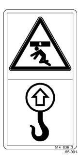
Only use the marked points to lift the machine. Never stand in the danger area or underneath a suspended load.
