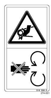
Do not open or remove the protective devices while the engine is running.
