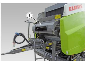
The net box can be fitted with a cover (1), as an option, which is designed to prevent crop accumulating on the net roller and tying device.
