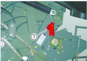
Refit the unblocking key (1) into the tensioning arm tube.
