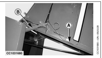
A-Lock device control lever
