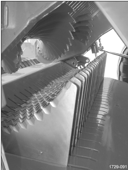
Figure 55 (Pictures from open bottom door) Knives in cutting position
