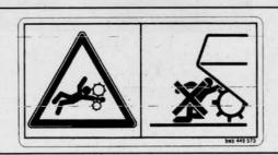
Never reach into pick-up area as long as tractor engine is running with PTO connected.
